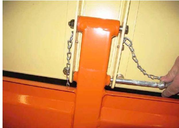
11. Secure Pins in place with Safety Pins.
