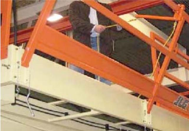
8. When rail is fully lowered, pull the bottom portion of the rope tight to release the Tool's Rail Clamp from the machine.
